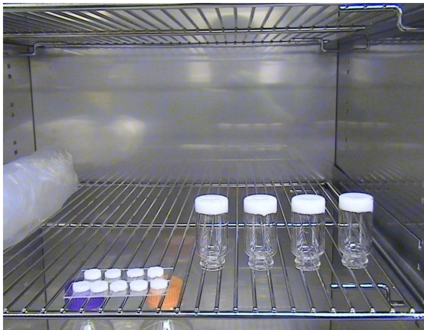
Figure 15 - Porous scaffolds drying inside oven at 40° Celsius.
